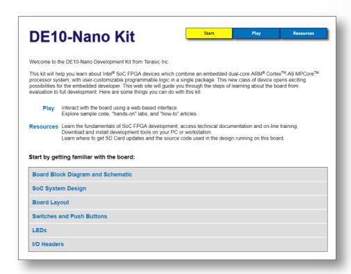
Users can connect the DE10-Nano to a computer via the micro USB cable and interact with the hardware through the website served by the board.
